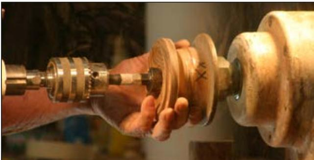
**Step 11:** (To create a “through finial”) Using a forstner bit, drill a hole into the lid. The hole should be the same diameter as the blank for the finial.
