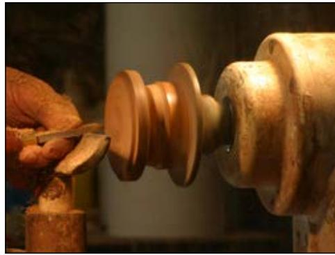
**Step 8:** Cut the bevel into the bottom of the lid. This should match the opening that you left in the top of the bowl. Tip — Test fit the bowl bottom to the bevel cut in the top (shown above right) or use calipers to measure the bevel against the opening.
