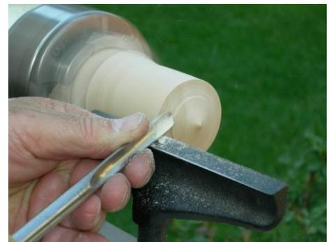
5. **Form the upper surface** with the spindle gouge. Additional detail (chatter-work, colored markers) may be added to this surface. *Cut away more of the bulkwood on the left side as you proceed, to **AVOID A CATCH**.* This would be a good time to sand and finish this surface
