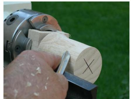
4. **Form the bottom** of the spin top. Low profile tops seem to spin longer. Start the cut about 3/8 of an inch from the face. Slowly cut down to the center. Do not force the gouge into the wood. At this point, decoration in the form of “chatter-work” or colored pens can be used to enhance the look of the top. This would be a good time to sand and finish this surface. Do not sand the tip.
