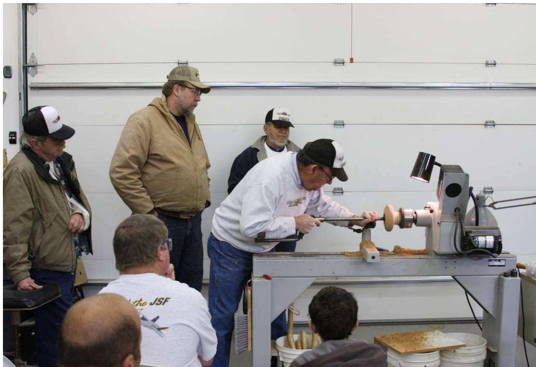
Here Dan is tackling the task of hollowing the vessel using an arm brace and a specially shaped square tool bit. This is always the scary part for most wood turners but Dan had several members try their hand at it and some of our experienced members contributed their techniques
