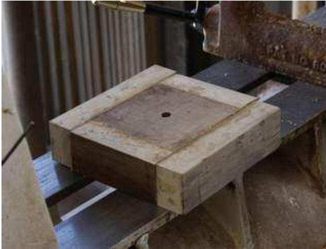
One of the keys to making the box is to start with a very square blank with sacrificial wood glued to the out sides. For this demo Martin used brown paper between the pieces to make it easier to separate later
