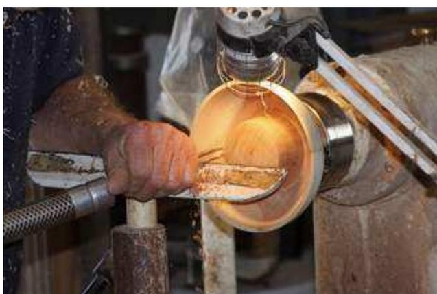
The inside is next and it helps to be careful with the bowl gouge since the inside curves change direction. You have to turn "downhill" and not go past the bottom while turning either side.
