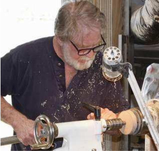
The last step is the lid. You can make it out of contrasting wood if you like. Don't forget to turn a slight curve in the inside of the lid to match the top of the box.
