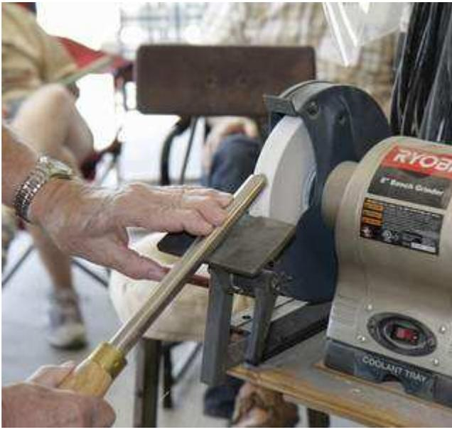
There are many ways to sharpening bowl gouges and get different profiles. Here Les demonstrates how to grind back the wings to get a sweptback profile on a gouge. He starts by grinding back the sides with the gauge upside down and flat on the grinder table. The turn it over and grind the bevel. Lots of our members use the One Way Wolverine sharpening guides on there grinder like this picture of Corky's
