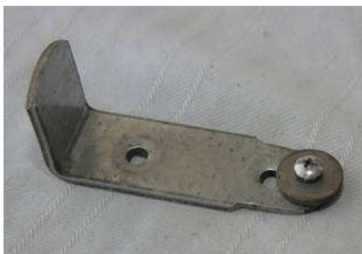
This is a picture of Corky's holder for the small scraper blades that we all use for hollowing the inside of hollow shapes. Corky just screw the blade to a flat piece of steel with a threaded hole on one end and a bent up section on the other. You hold onto the bent up end and the other lays flat on the grinder table. A great idea for a difficult job.
