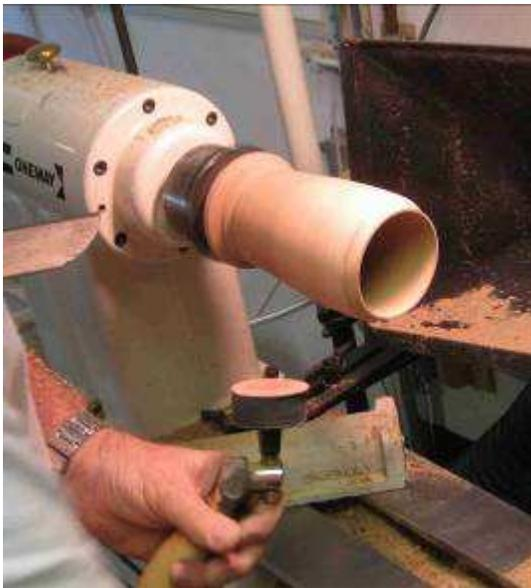
After turning a pleasing shape on the outside its time for some sanding
