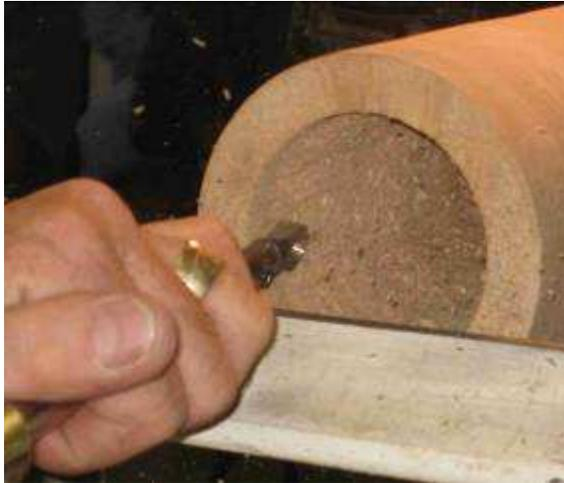
Here's a close-up of the ring tool. Robert had a small cone shaped grinding tool that fits in a router to sharpen the tool. He also uses a special holder to hold the ring square to the sharpening tool. Cool!
