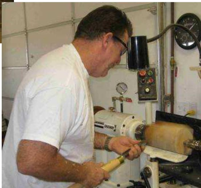
Robert had a lot of useful tips and tricks for turning. Here he is using a Max-Min gage he made the shows the maximum and minimum of the jaws on his chuck. He just has to turn a tenon whose diameter is in-between the two. Later you will need to hold the piece in the chuck using the tenon to bore out the inside for the liner.
