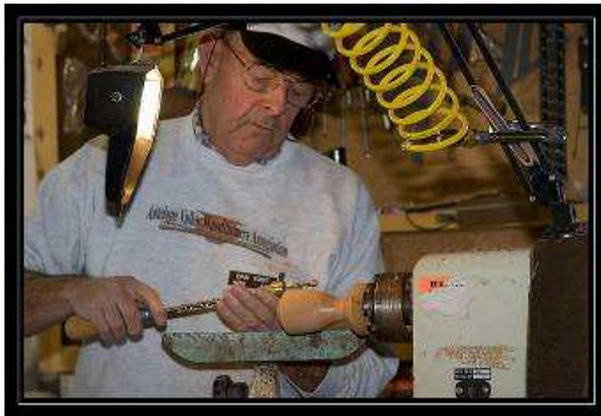
After turning the outside shape Dan gets ready to start the inside by using a drill with a stop to bore a hole.
