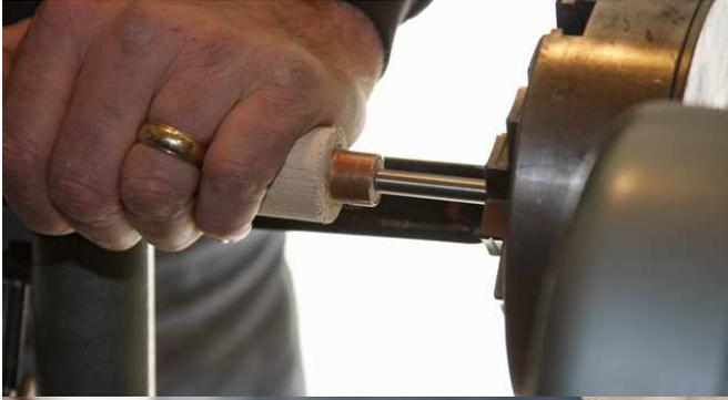
With the rod in the chuck use the tailstock to press the handle onto the rod
