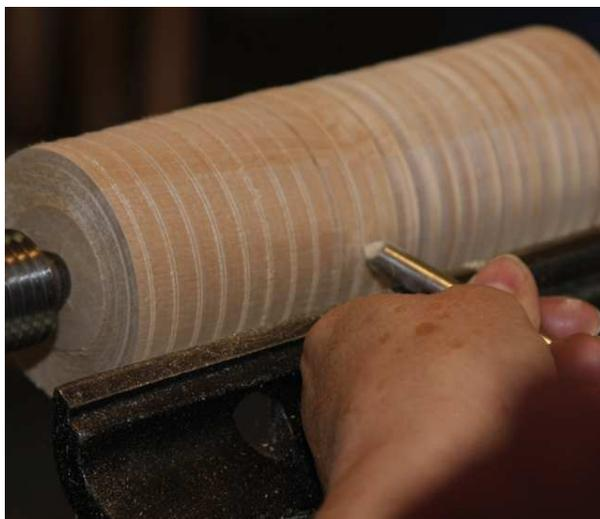
Using the pyramid tool you can create the notch for the start of the bead and turn the bead without fear of a catch.
