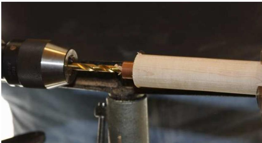
Now drill a hole .03 smaller than the diameter of the rod you cut off from the reamer. This will create a tight press fit so no glue is necessary. The ferrule keeps the handle from splitting
