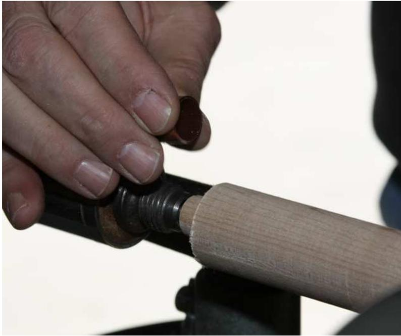
After turning a blank round, you make a tenon on one end that will fit a ferrule that is made from a piece of copper pipe
