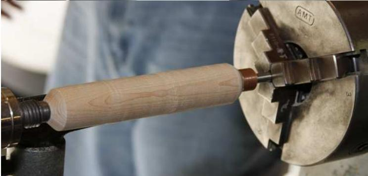
Turn the outside of the handle while its held in the chuck
