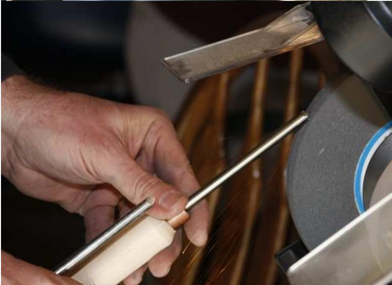
Sharpen the tool by grinding three sides to an equal angle. This is easier if you mark the opposite sides using a marker, then keep each mark up while grinding.
