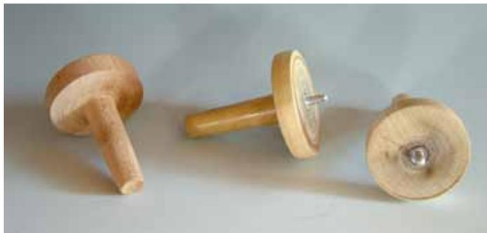
When inserting the slip clutch into the lathe for the first time, hold it from spinning while the lathe is turning to allow the taper to find center. Try to get the metal point (I make my points from six penny nails.) dead-centered in the clutch. Cut the nail about 2 inches long and allow 1/2 inch to extend out.
