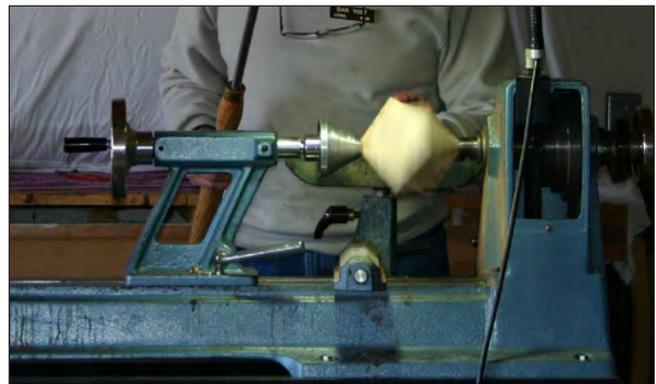
**Step 2:** Turn the outside shape of the bowl nearest to the headstock. Cut a tenon for mounting in a chuck.
