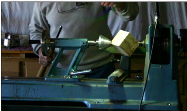
**Step 1:** Mount a perfectly square cube between the lathe headstock and tailstock. Make sure the starting block is exactly square, or the three corners will not be equal.
