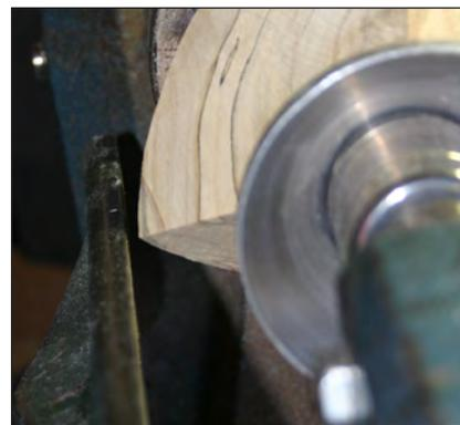
**Step 4:** Check the runout (the distance between each corner and the tool rest). The distance should be equal for each of the three corners.
