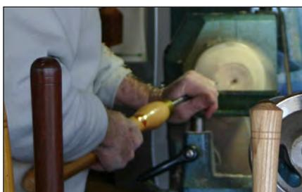
**Step 5:** Pull back the tailstock, turn off the outside corner, then core out the inside of the bowl as normal.
