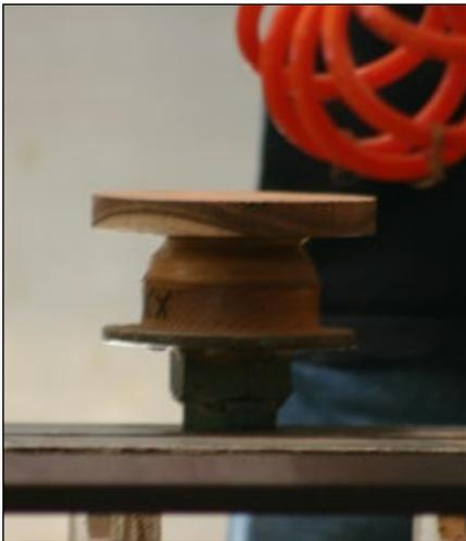
**Step 1:** Cut off the box top from the overall blank. Use a band saw before the blank is mounted to the lathe, or use a parting tool if mounted on the lathe. You will also need a separate finial blank, which can be a contrasting wood (see Step 11.)
