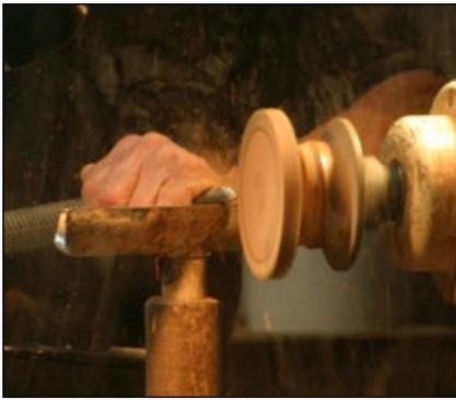
**Step 7:** Mark the bevel diameter (the same as the opening in the bowl bottom) with a pencil.
