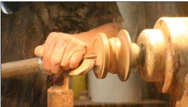
**Step 9:** Finish the inside of the lid as desired — add some curving should be applied so the inside of the bowl lid matches the contour you will create on the outside of the lid.
