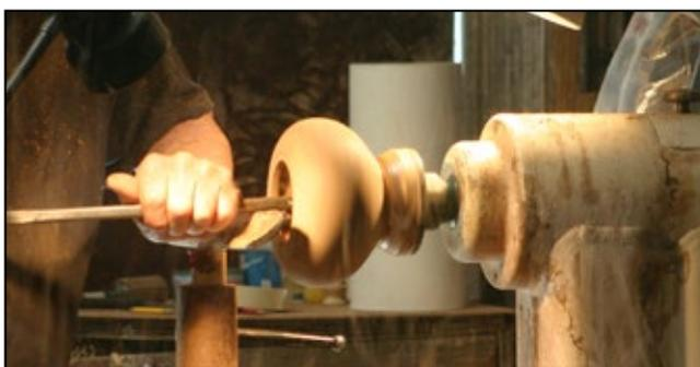
**Step 5:** Use hollowing tools to complete the inside of the bowl.
