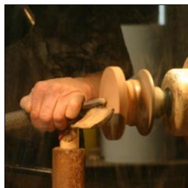
**Step 6:** Mount the lid blank on the lathe. Use turning tools to smooth and balance the inside of the lid blank. The lid blank should also be mounted to a waste block.
