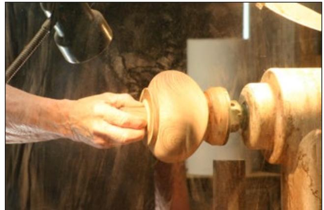
**Step 12:** Mount the bowl blank back onto the lathe. Place the lid on the bowl and turn the lid outside and finial blank to the desired shape. You can use the tail stock to hold the finial/lid in place, or tape the lid to the bowl in place and finish the piece.
