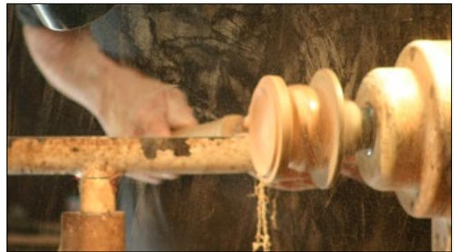
**Step 10:** Turn the outer edge of the lid to the finished size.
