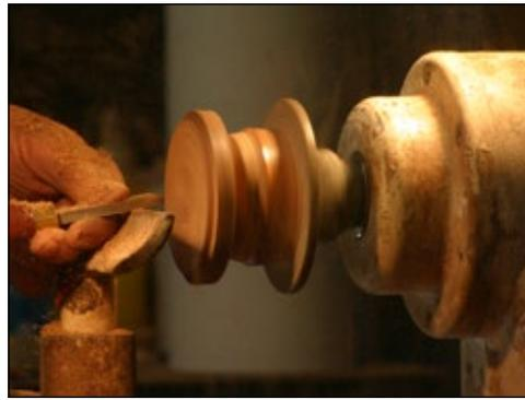
**Step 8:** Cut the bevel into the bottom of the lid. This should match the opening that you left in the top of the bowl. Tip — Test fit the bowl bottom to the bevel cut in the top (shown above right) or use calipers to measure the bevel against the opening.
