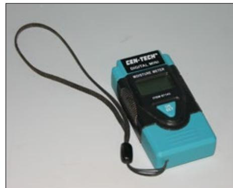
A moisture meter like this one can be used to measure the MC of a piece of wood.
