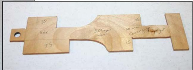
Simple wooden gauges offer a quick way to determine the appropriate size tenon. Steve has created a different template for each set of chuck jaws since the different sizes and configurations allow different optimum tenon sizes.
