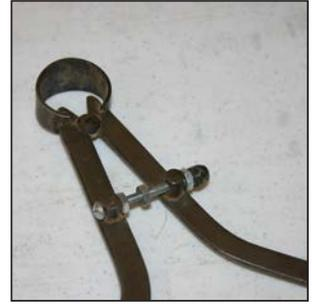
By replacing the standard mechanism (left) with a bolt and a few nuts (right), Steve has created a set of calipers that can be adjusted to function almost as a thickness guage. Positioning the nut in between the caliper arms forces the caliper to stop closing at a specific thickness — for example, the thickness of a hollowform wall at a specific point.
