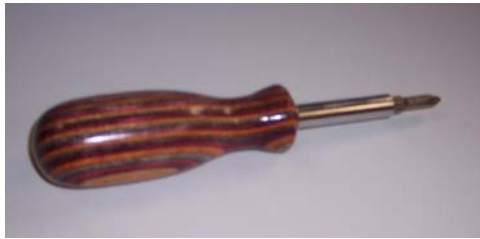
"Junk Drawer" (i.e. four and one) screwdriver Colorwood; CA glue finish Bob Clark
